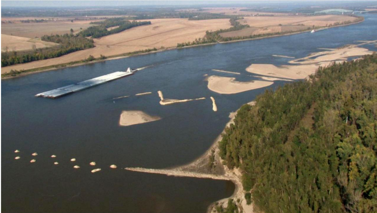
Use of dikes and revetments on the Mississippi River [1]
